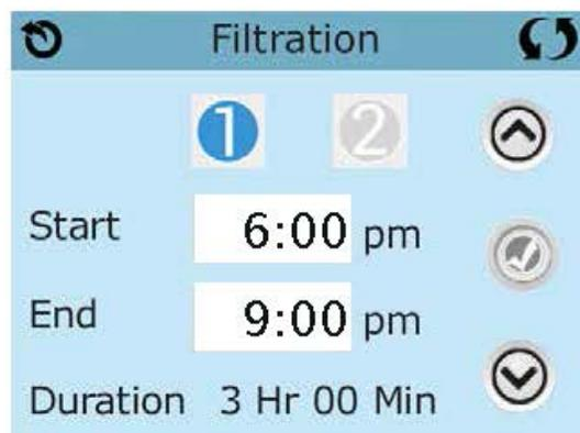
Viewing Filter 1 while Filter 2 is OFF:
